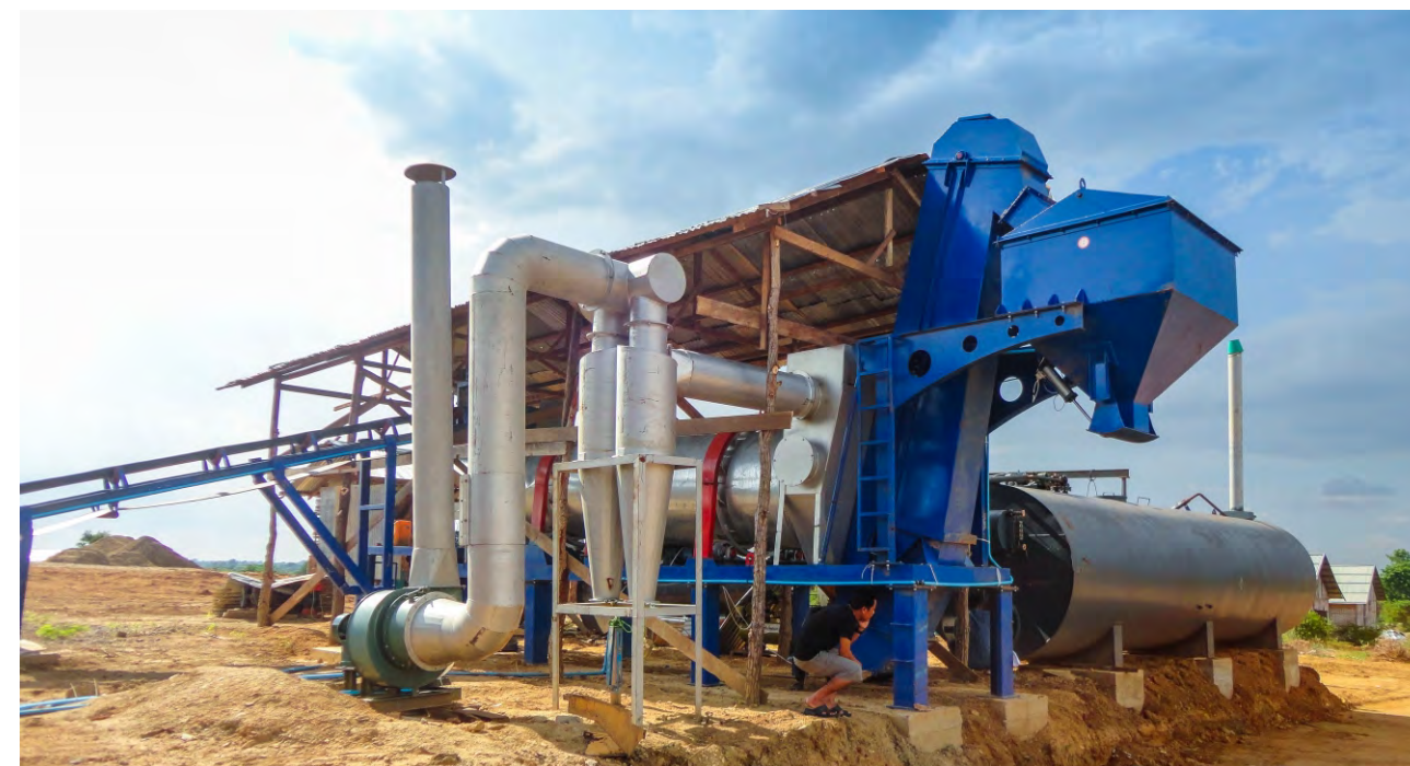
DAP40 📍 Myanmar 🚚 40T/H DAP40 Drum mix asphalt plant in Myanmar
