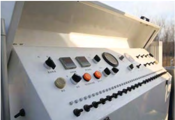
Control panel at the end of the distributor truck, enable manual operation
