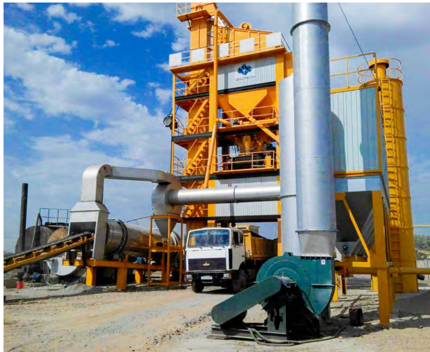
BAP80 📍 Uzbekistan 🚚 80T/H BAP80 Batch mix asphalt plant in Uzbekistan
