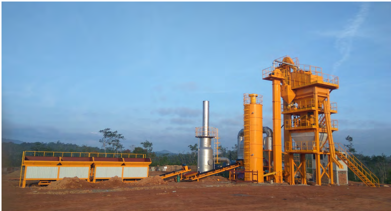
BAP60 📍 Myanmar 🚚 60T/H BAP60 Asphalt batch mix plant in Myanmar
