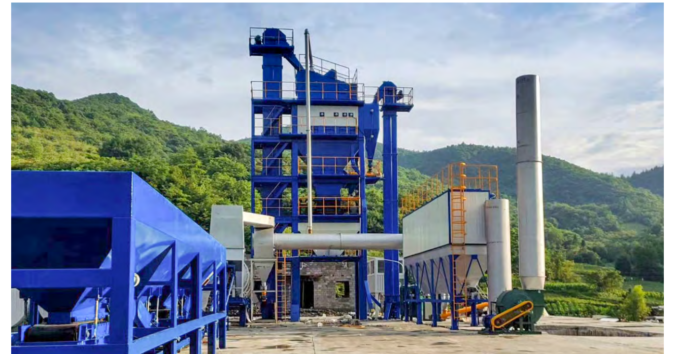
BAP80 📍 Zambia 🚚 80T/H 80t/h Batch mix asphalt plant in Zambia
