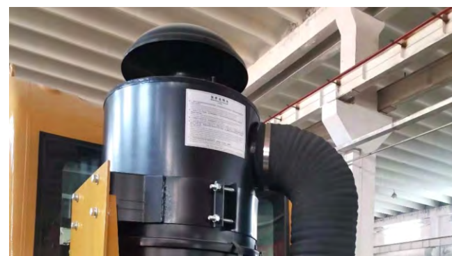
Two-stage filtration to prevent dust from entering the engine
