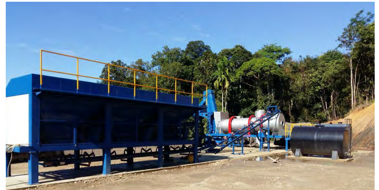
DAP20 📍 Malaysia 🚚 20T/H DAP20 drum mix asphalt plant in Malaysia
